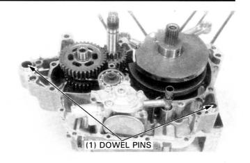
Assemble the right and left crankcases being careful to align the dowel pins and shafts.
