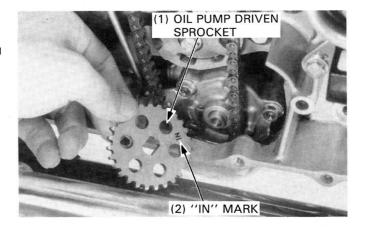
Apply locking agent to the threads of the driven sprocket mounting bolt and tighten it with the washer to the specified torque.
