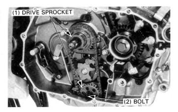
Align the grooves in the clutch outer with the bosses on the oil pump drive sprocket while turning the sprocket with the chain and pushing the clutch outer onto the shaft.
