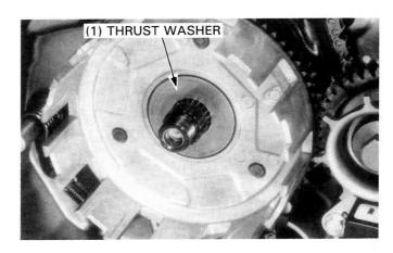
Install the pressure plate, clutch discs B, plates and disc A in the clutch outer.
