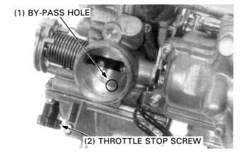
Align the front cylinder carburetor throttle valve with the bypass hole edge by turning the synchronization adjusting screw.
