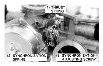
Separate the carburetors by removing the two attaching screws.
