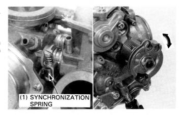
Turn the throttle stop screw to align the rear cylinder carburetor throttle valve with the edge of the by-pass hole.
