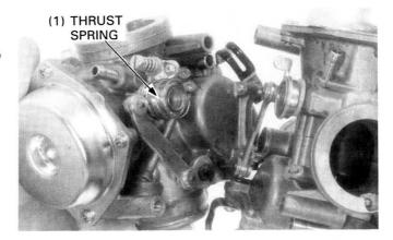
Install the synchronization spring and synchronization adjusting screw.
