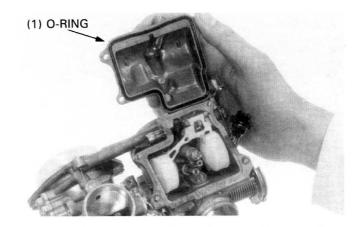
Install the float chamber and tighten the screws securely.
