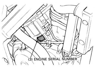
The engine serial number is stamped on the right crankcase below the rear cylinder.
