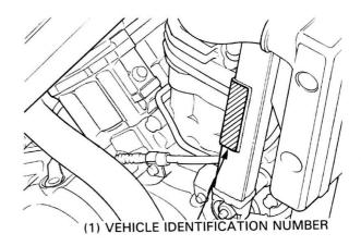
The vehicle identification number (VIN) is attached to the right side of the down tube.
