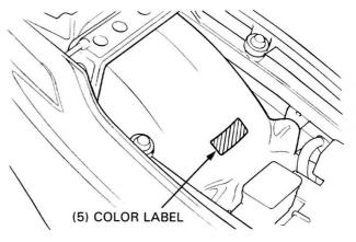
The color label is attached to the rear fender under the
