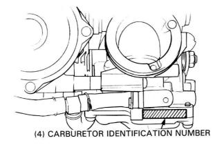
The carburetor identification numbers are on the carburetor body intake side.
