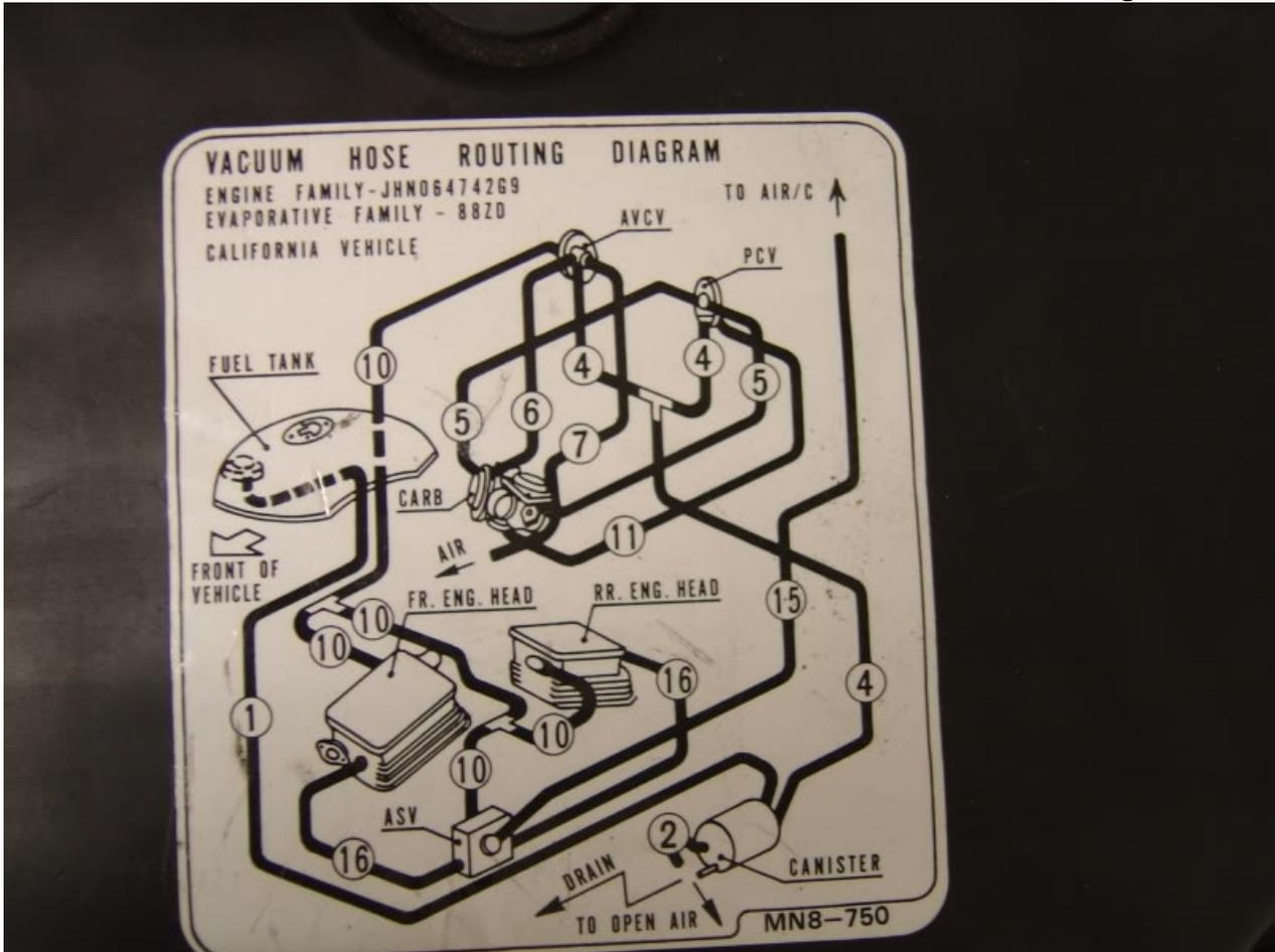
1) Cap all of the smog control related fittings on the side of the carburetor that connects to the engine.
