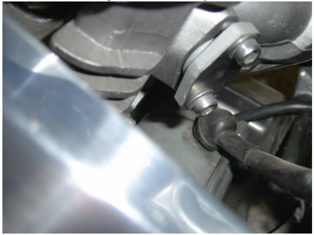
The metal tubes No 16 in first diagram will need some block off plates made like this
