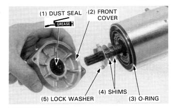
Align index marks of the front cover, case and rear cover as shown.
