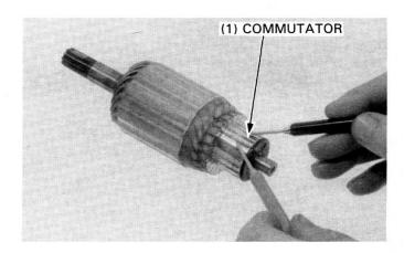
Check for continuity between individual commutator bars and the armature shaft.
