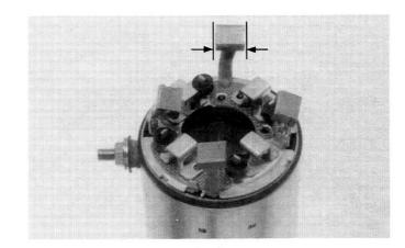
Check for continuity from the cable terminal to the motor case and from the cable terminal to the brush wire (black).
