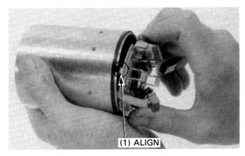
Install the armature in the case. Set the brush springs.
