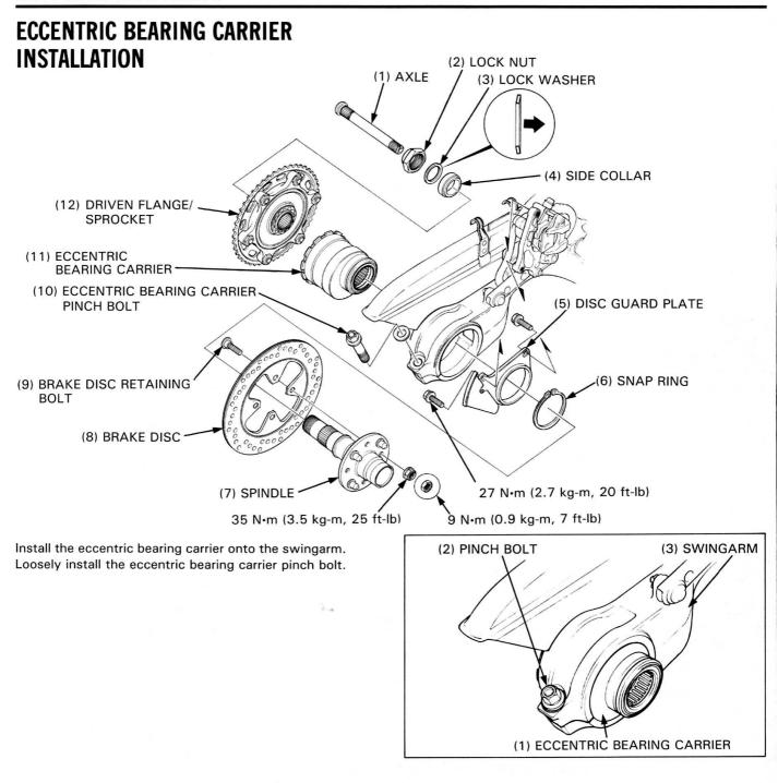
Install the brake disc guard plate onto the eccentric bearing carrier by using the snap ring.
